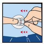
6. Place a finger on the cannula housing while pushing the site connector straight in until you hear a "click".
